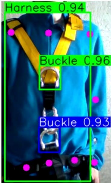
Figure 4: Harness with two buckles, one at sternum level (green) one too low (blue)
