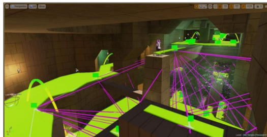
FIGURE – Unreal Tournament's series bots use a pathnode system embedded in the map to navigate
